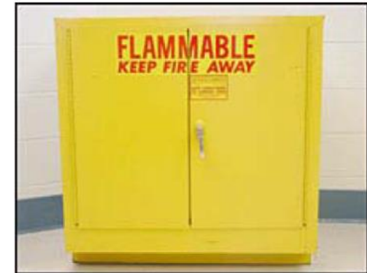
Store flammable combustible liquids in rated flammable cabinets.
