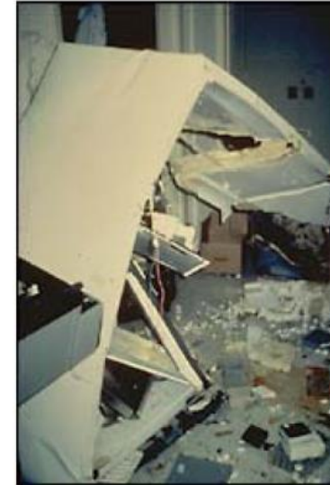
Explosion of residential type fridge improperly used for flammable storage.
